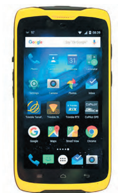
▲ Figure 1: Trimble TDC100 handheld data collector combines smartphone and GNSS technology.
