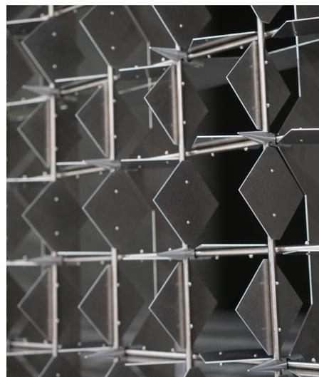
**Figure 3.** Close up of the active grid flaps, axes and intersections.
