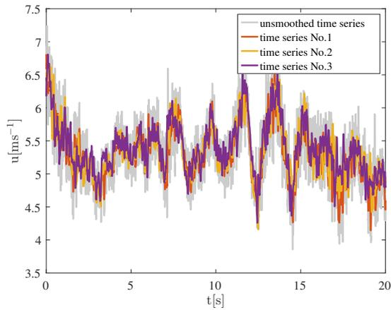
**Figure 5.** Wind speed time series behind the active grid using the LiDAR excitation protocol
