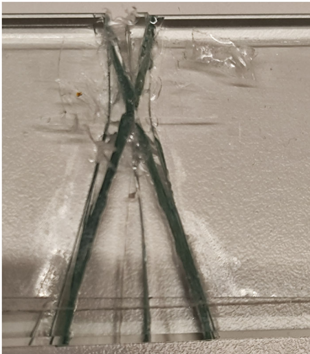
Fig. 11 Surface or X failure, specimen B1
