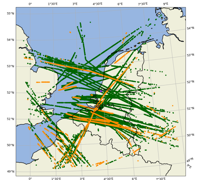
Fig. 9. Aircraft trajectories: training set (green) and test set (orange), as measured by an ADS-B receiver located at Delft, from 11:30 until 12:30 on 10/01/2018, FL 340-380 [32]. (via Cartopy [21])
