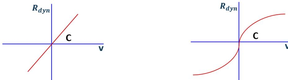
Figure 16: Soil damping models with linear (left) and exponential (right) relation to pile velocity
