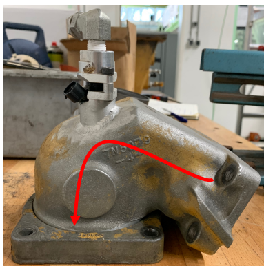
Figure 2.1: Airflow through inlet air receiver
