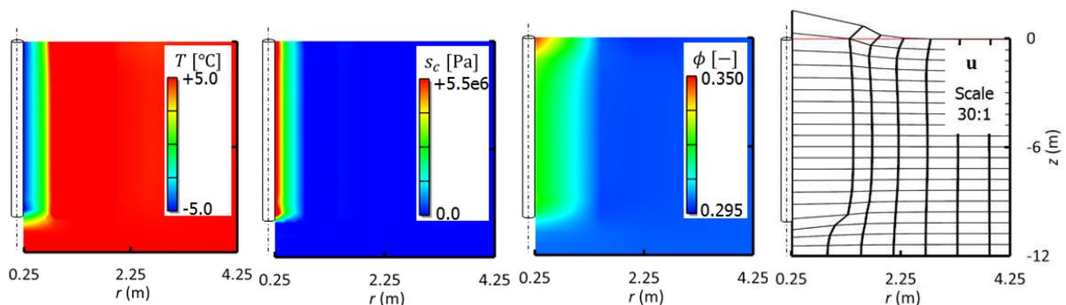
Fig.2 Temperature, cryosuction, porosity and deformation during freezing.
