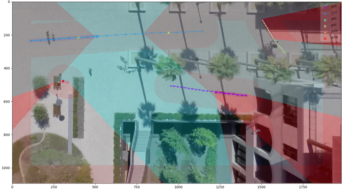
(b) An agent is randomly selected as the "target" for occlusion simulation. Eligible "target" candidates must be moving, the probability of an agent being selected as target is proportional to their distance travelled over t \in \{-T_{\text{obs}}; T_{\text{pred}}\} . The blue region, B_{\text{ego}} , is defined as the intersection of the visibility polygons for the first and last trajectory points of the target agent, with the past trajectories of other agents acting as visibility constraints, to prevent cases where an agent might lie between the target and p_{\text{ego}} . Two yellow points in the target's trajectory are randomly sampled as the first and last non-occluded points (one in [-T_{\text{obs}}; 0] , one in [1; T_{\text{pred}}] ). Mutually opposite wedge shaped red regions are defined from those first and last non-occluded points, and are added to R_{\text{ego}} , in order to minimize risk of aligning the ego directly with the trajectory of the target.
