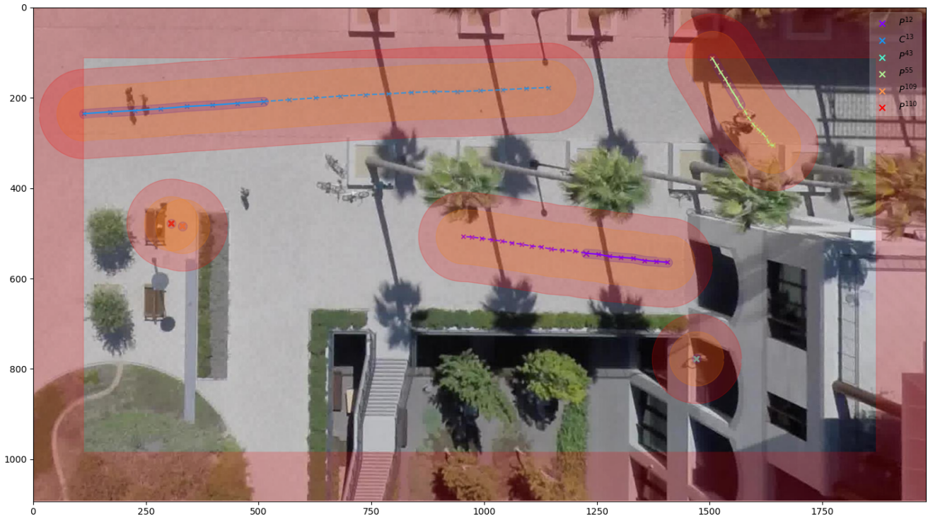
(a) The red regions, R_{\text{ego}} , restrict the placement of the virtual ego p_{\text{ego}} within the workspace. They correspond to the regions of points within a distance d_R from agent's complete trajectories over t \in \{-T_{\text{obs}}; T_{\text{pred}}\} , or a distance d_B from the boundaries of the scene. Similarly, orange regions circumvent agents' trajectories, with delimiting distance factor d_O , in order to limit the positioning of the points defining W_{\text{occl}} . We set d_R > d_O , in order to ensure that some free space exists between ego and trajectories, facilitating the placement of W_{\text{occl}} .
