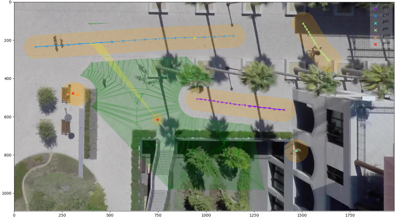
(c) The candidate region for placement of p_{\text{ego}} (in green) is defined as B_{\text{ego}} - R_{\text{ego}} . A random point is sampled from this region. This point will be the virtual ego, p_{\text{ego}} (the red circle). A small region around p_{\text{ego}} is added to O_{\text{occl}} , ensuring a minimal distance d_{\text{ego, occl}} between the occluder and the ego. The triangular candidate region for placement of p_{\text{occl}, 1} is obtained using p_{\text{ego}} , the last observed point (in yellow), and the first unobserved point.
