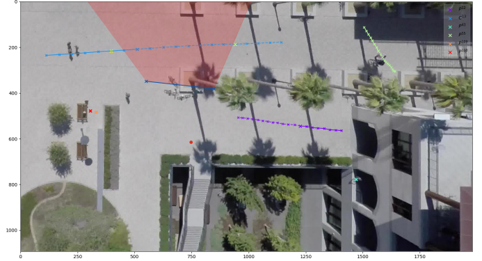
Fig. 5: An example of a scene generated from our occlusion simulator. The red area constitutes W_O , and is obtained from computing the visibility polygon of the virtual ego, obstructed by a virtual occluder (respectively shown as a red dot located below W_O , and a dark blue segment at its lower boundary). Trajectories are shown as sequences of points: full lines connect trajectory points which are in the past, and dashed lines indicate the future part of the trajectory.
