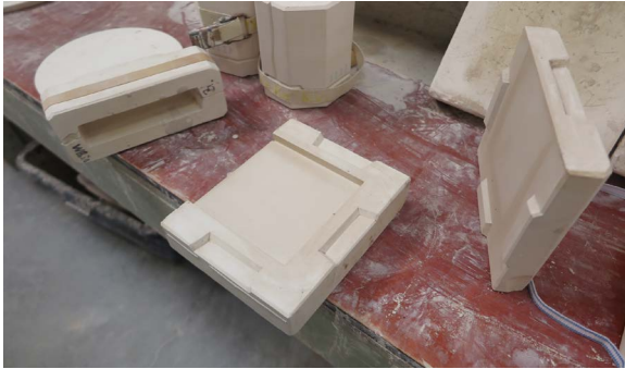
32. Tiles are cast in this 2-part mold
