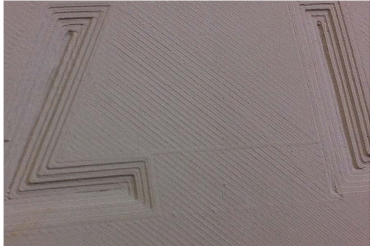
62. Unspunged clay body based on an FDM PLA-print
