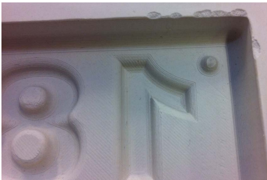
49. Mold chipping on edge and print relief
