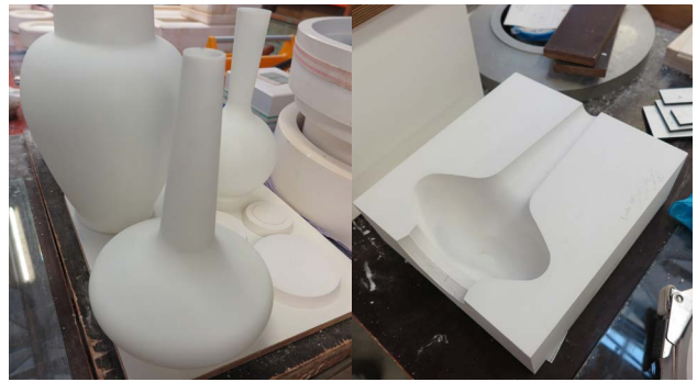
33. Vase and one of its mold parts. While a vertically oriented 2-part mold would have required less sponging, the shape is still cut up horizontally, to reduce risk of breaking the clay body.
