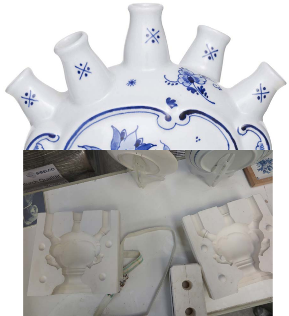
34. Similar looking features with different production methods: this shape has 3 cast sprouts, and 2 garnished sprouts.
