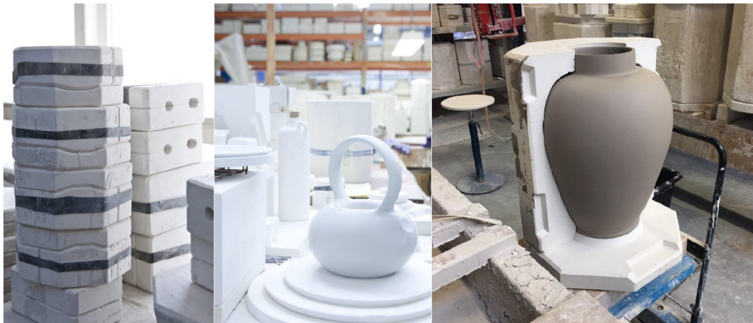
image / figure 1: Molds and half-fabricates at Royal Delft (image courtesy of Royal Delft)
