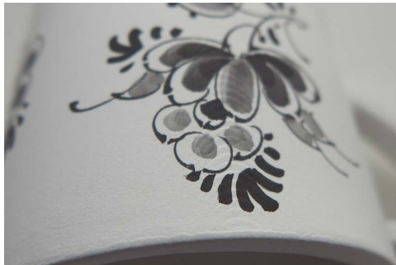
47. Relief is not covered by engobe-layer, still visible on biscuit
