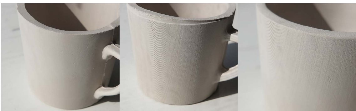
39. A3D printed mother mold produces a rougher shape (middle), but successful sponging is possible (right)
