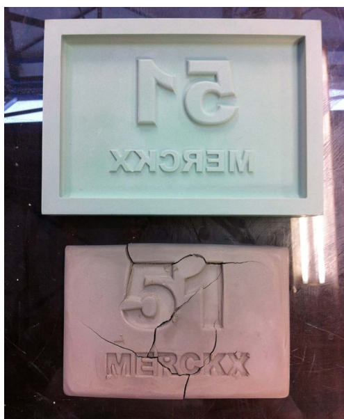
55. Obumodulan pressing mold with cracked clay body
