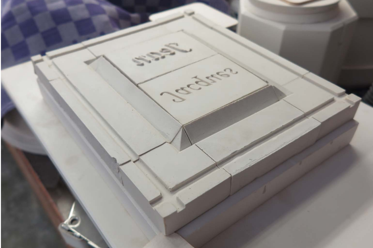
82. Visible gaps between mold edges and inserts
