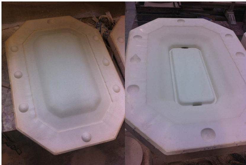
71. Bottom (left) and top (right) mold part of a large plate
