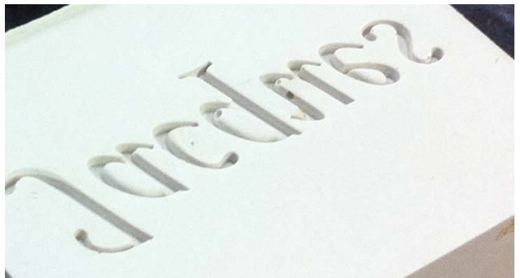
63. Plaster mold part based on an SLA-print
