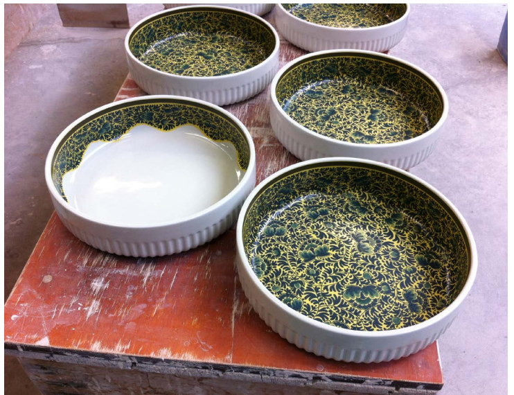
27. Fully and partially applied transfers
