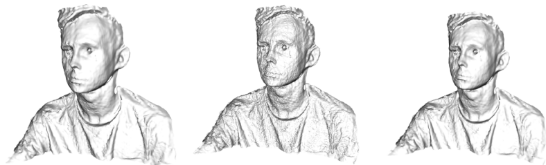
[Figure 26] Result after applying an average filter (Left), a Taubin filter (Middle) and both average and Taubin filters (right).
