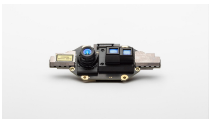
[Figure 40] Azure Kinect DK (top) and internal sensor hub of Azure Kinect DK (bottom).
