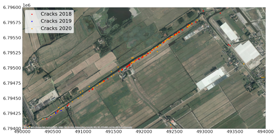
FIGURE 4.10: Zoomed in plot of the Berkelsche Zweth, where the cracks registered in the different years are given.
