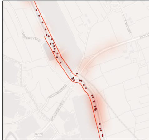
FIGURE 8.6: The map shows the Molenlaan, where the cracks are plotted as red dots, the hazardous areas as the heat maps and the lists as the red lines.
