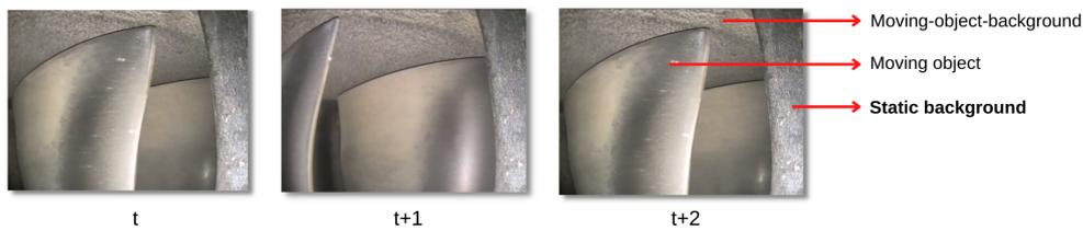
**Figure 2.2:** Video frames from borescope inspection at different time intervals. We split the video into three parts namely a static background, moving-object-background and moving object.
