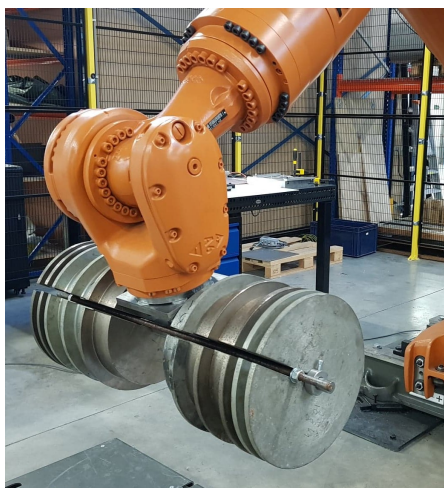
Figure 2-6: Custom barbell tool mounted on the KUKA robot
