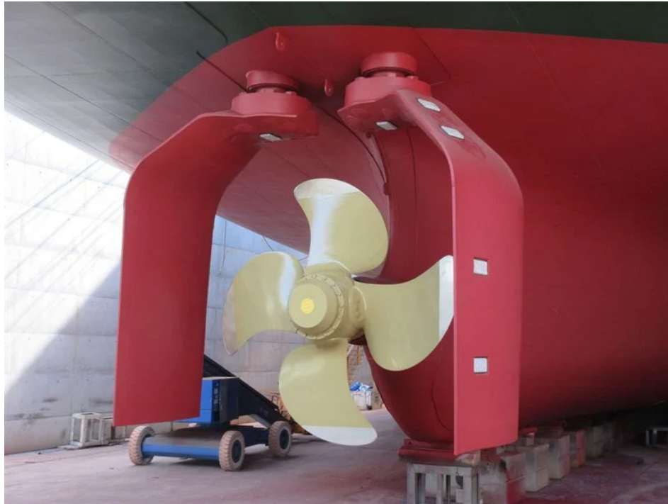
Figure 1.1: Example of a gate rudder system (GRS) installed on a Japanese domestic container vessel, Shigenobu. Credit: Yamanaka Shipbuilding.
