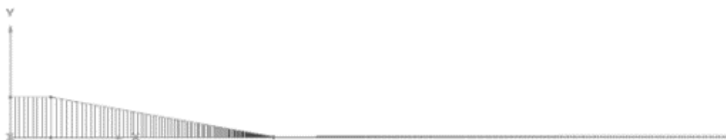
Figure B.2: Nozzle with one dimensional mesh. Finer mesh is observed near the throat. This nozzle is used for the reference case where supersonic outflow is observed for nozzle 2 [2].
