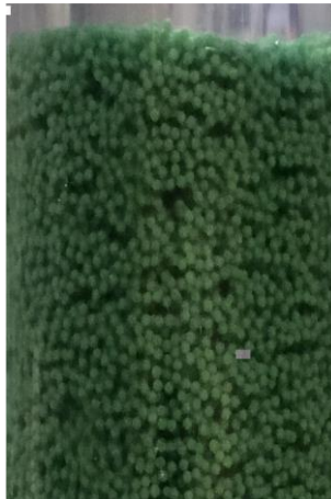
Figure 56 Fluidised glass beads in water at relatively low fluidisation (1.5 mm 12 °C, 25 mm/s)
