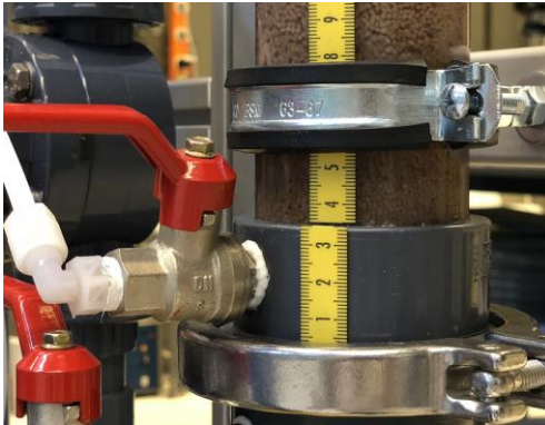
Figure 32 Lowest section of the expansion column with the lowest tab and the grid at the bottom
