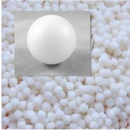
Nylon balls (DitHolland) d_p = 3.0 mm
