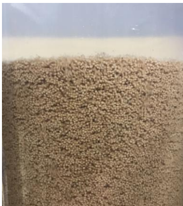
Figure 121 Single fraction experiment 0.9-1.0 mm calcite pellets
