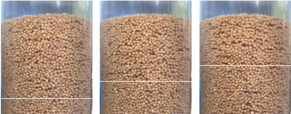
Figure 66 Sequence of 1.4-1.7 mm calcite pellets in a 57 mm column. Dark zones are caused by local pockets of water, v_s = 25 mm/s, \langle \epsilon \rangle = 0.50 m 3 /m 3 , average interstitial fluid velocity 50 mm/s. White lines represent the progression of waves of voids moving up at 50 mm/s. The time interval between images is 0.17 s, corresponding to 8.5 mm or 5.5 particle diameters. The wave progression can be seen more clearly on the provided video material (Kramer et al., 2020e; Kramer et al., 2020h).
