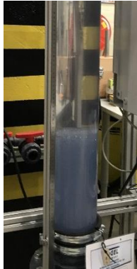
Figure 116 3 mm glass beads (Boom lab) at v_s = 240 m/h
