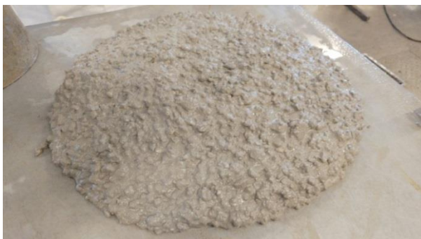
Fig.1 Slump test of optimized concrete mixture
