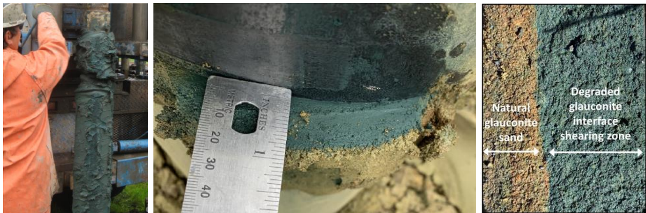
Figure 2.20. Glauconite Sand Degradation due to Drilling and Pile Driving from Westgate et al. (2023; 2024)
