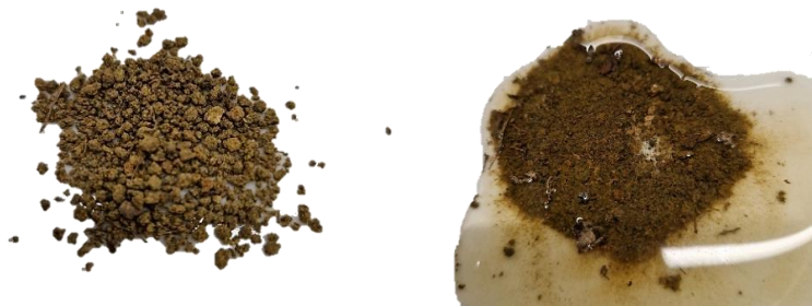
Figure 4.7. Oven-Dried Leuven Sand Clumps Breaking Down with Wetting
