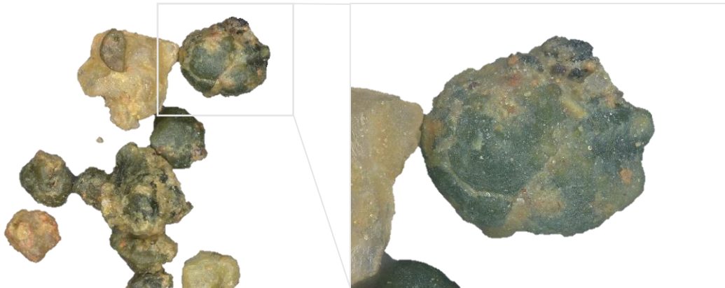
Figure 4.3. Digital Microscope Images of Glauconitic Sand Particles without the 1 M HCl Pre-treatment
