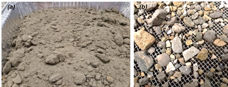
Figure 3.5. Antwerp Sand Sample: (a) Full Fraction and (b) Gravel Fraction
