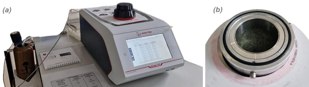
Figure 4.10. (a) Gas Pycnometer and (b) Medium Load Cell
