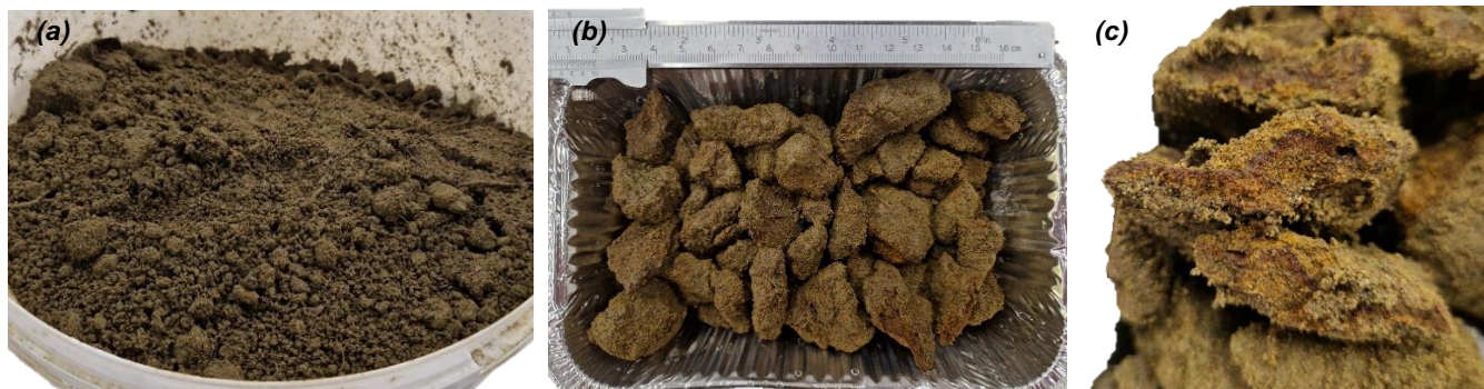
Figure 3.4. Leuven Sand Sample: (a) Full Fraction and (b-c) Oxidized Agglomerates
