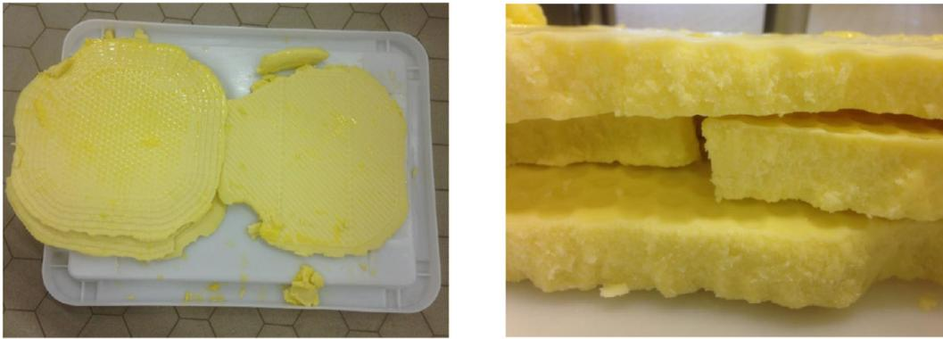
**FIGURE 4** Top view and side view of filter cakes produced in the pilot plant filter press. The membrane side is up. The thickness of the cakes is almost 25 mm [Color figure can be viewed at [wileyonlinelibrary.com](http://wileyonlinelibrary.com)]
