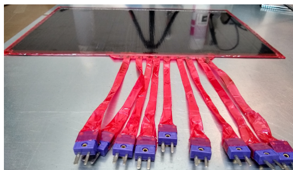
Figure 6.8: Isolation of thermocouple wires
