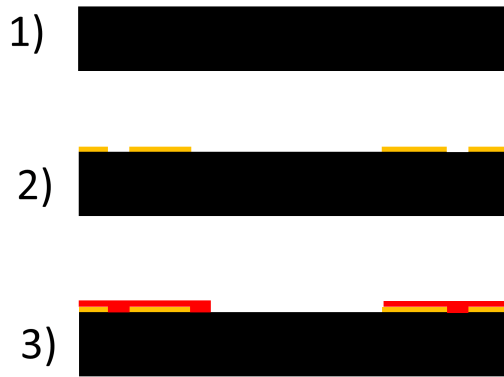
Figure 3.10: . Cross-section view of the flowchart for the silicon-based micropump and microfluidics, steps 1, 2, 3. Black: silicon, yellow: silicon oxide, red: photoresist.
