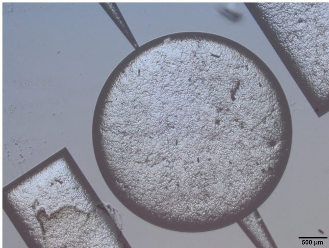
Figure 3.16: Close view of the pumping chamber after 2h30' of XeF 2 etch. The membrane could not be released.
