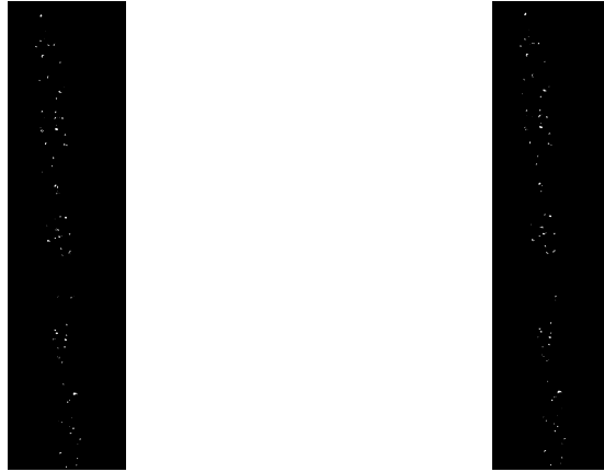
(a) Binarized image of the frame 71 (resulting of the background subtraction and thresholding, moving particles can be seen). (b) Binarized image of the frame 72 (resulting of the background subtraction and thresholding, moving particles can be seen).
