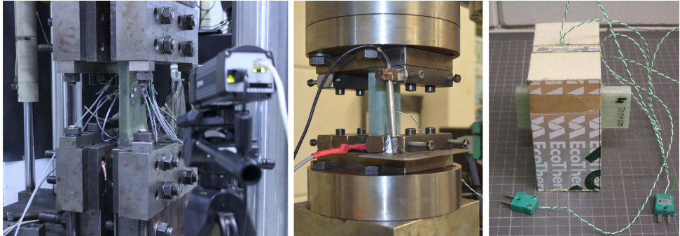
Figure 2.5: S77 coupons setup (left), 20 mm end-loaded coupons setup (middle), insulated end-loaded coupons setup (right).
