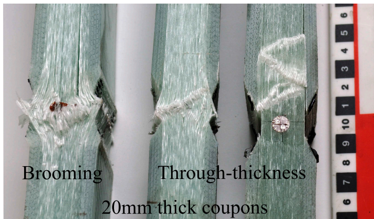
Figure 3.12: Failure modes photos in 20 mm thick coupons.
