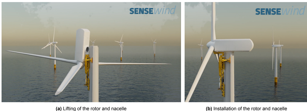
Figure 2.10: The SenseWind turbine mounted crane that can remove the rotor and nacelle assembly [37]
