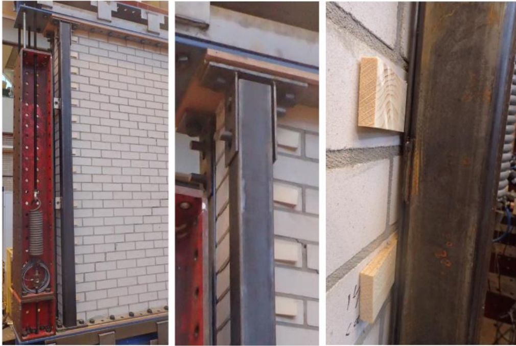
Figure 45: Lateral support system for OOP tests with detail of the applied wooden wedges (Ravenshorst & Messali, 2016b)
