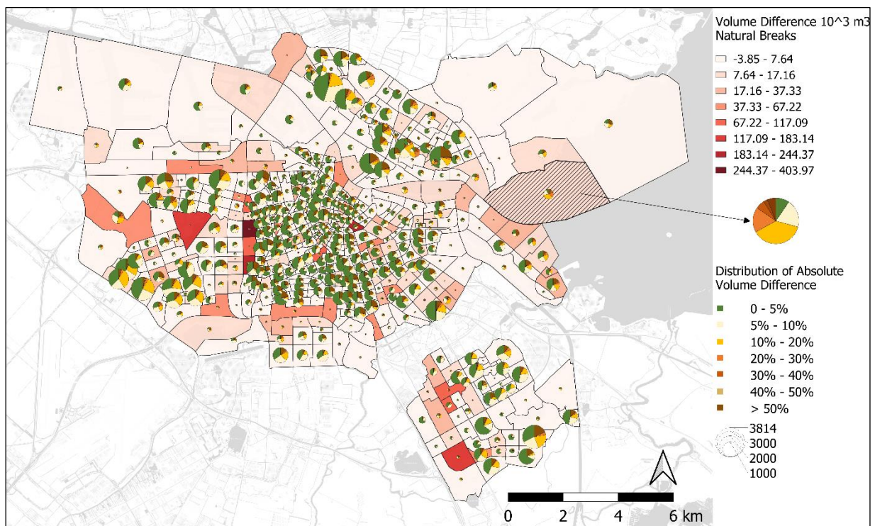
Figure 12. Distribution of volume differences between LoD22 and nDSM aggregated at neighbourhood level.
