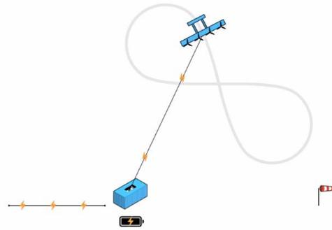
Figure 2.2: Fly gen AWE system in operation [10]
