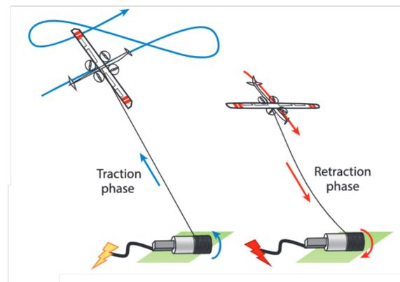
**Figure 2.5:** Fixed-wing ground gen system showing traction and retraction phase [9]
