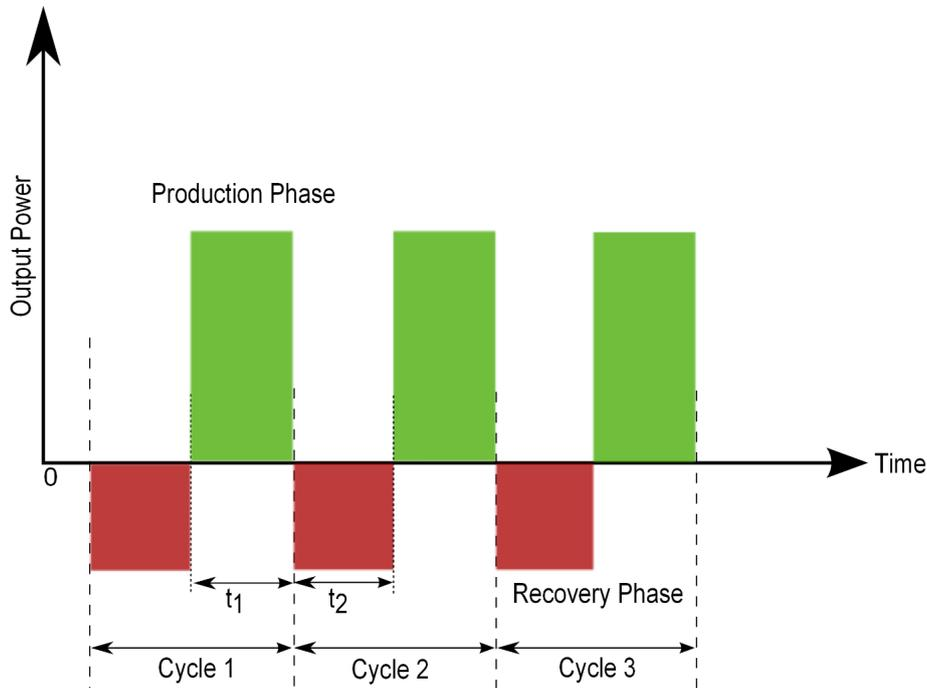
Figure 3.6: Plot of the power cycle for an AWE system [62]
