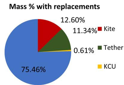
**Figure 3.14:** Pi chart showing mass share of components over the operational lifetime
