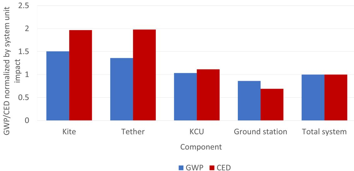
**Figure 3.23:** Mass specific impact of GWP and CED normalized by their respective specific system impact
