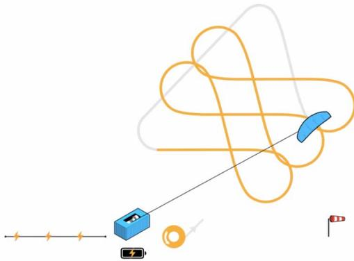
Figure 2.1: Ground gen pump AWE system in operation [10]
