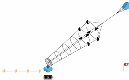
Figure 2.3: Ground gen rotary AWE system in operation [10]
