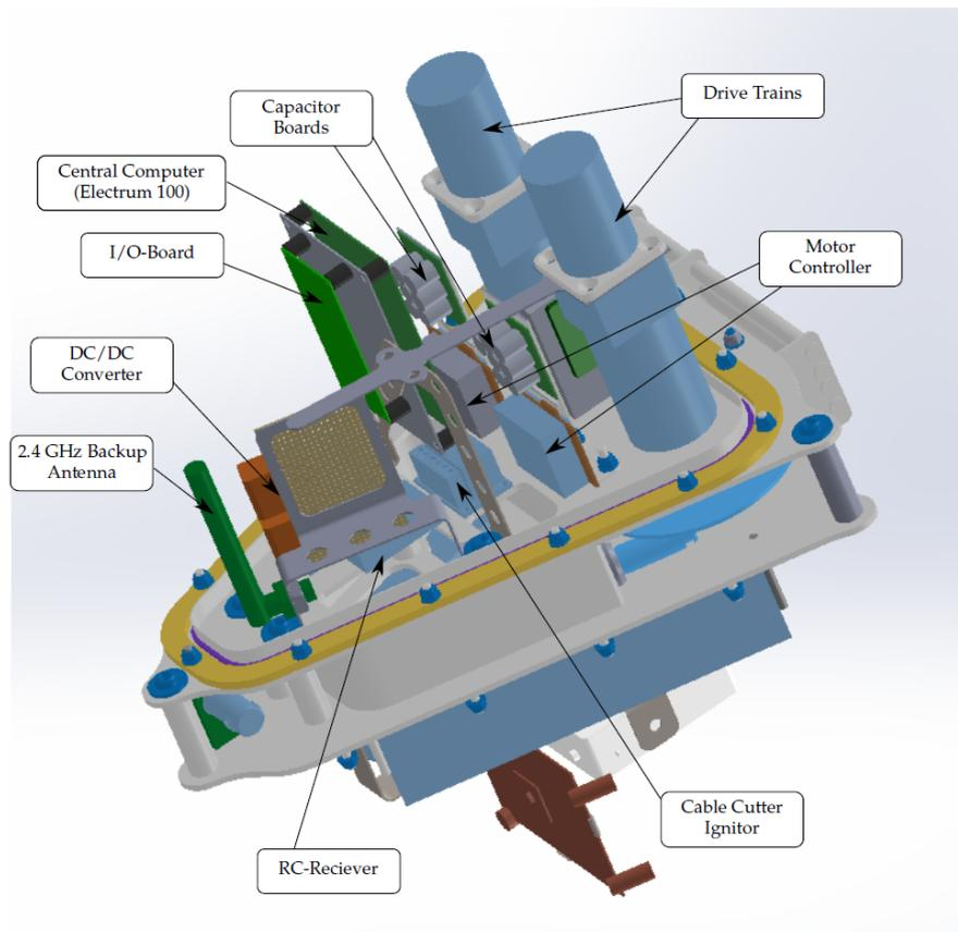
Figure 3.7: A CAD model showing different components within the KCU [65]
