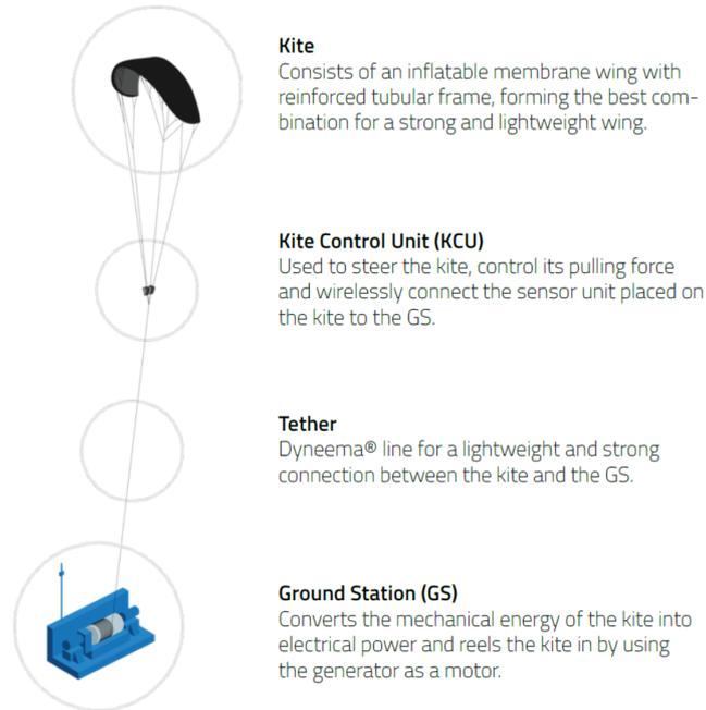
**Figure 3.2:** Diagram of Kitepower Falcon system with breakdown of main components [18]
