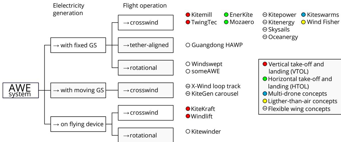
**Figure 2.6:** An overview of the different AWE technologies with relevant companies developing these [13].
