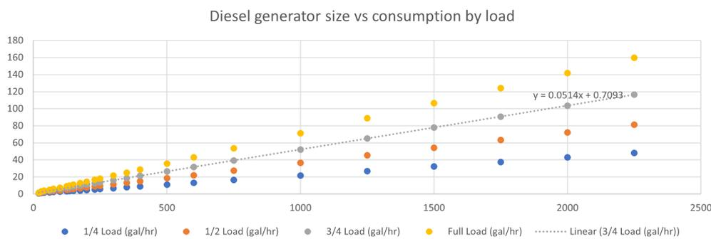
Figure 4.2: Plot of diesel fuel consumption against the generator size for different loads [80]
