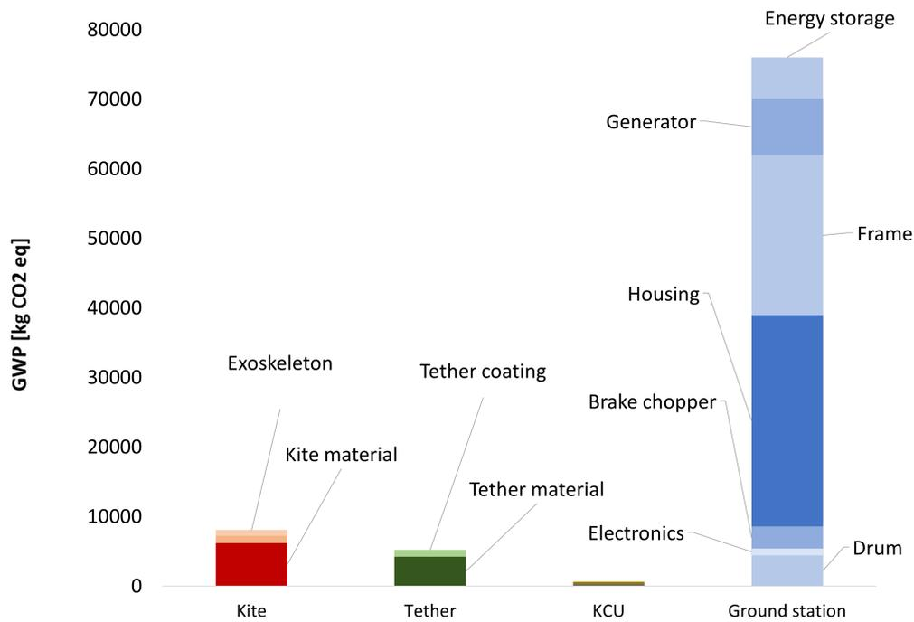
**Figure 3.16:** Plot showing the detailed GWP contribution of the AWE system
