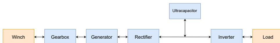
**Figure 3.8:** Block diagram showing the electrical drivetrain of the ground station using an ultracapacitor [66]
