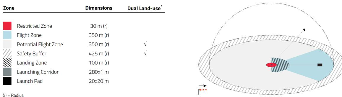
**Figure 3.9:** Operational zones of the Falcon system with legend [18]
