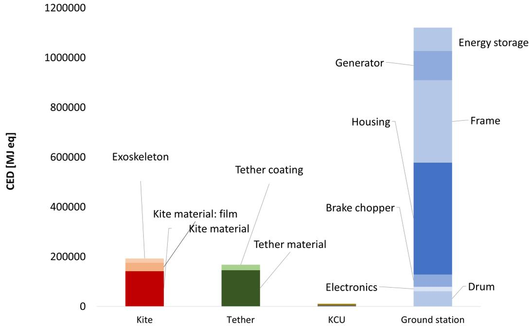
Figure 3.17: Plot showing the detailed CED contribution of the AWE system
