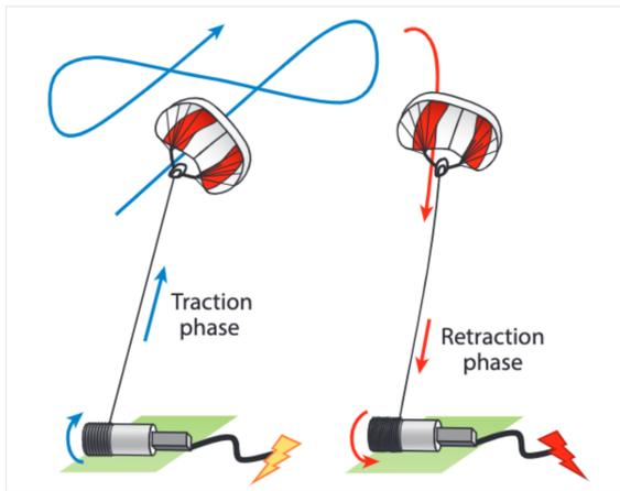
**Figure 2.4:** Soft-wing ground gen system showing traction and retraction phase [9]
