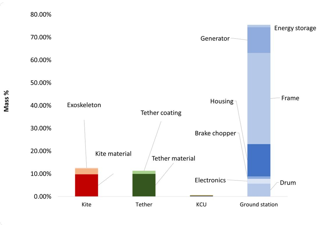
**Figure 3.15:** Plot showing the detailed mass % contribution of the AWE system
