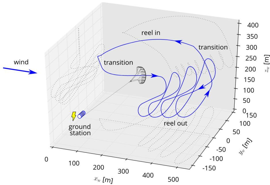
**Figure 3.5:** Plot showing the trajectory of the AWE system [61]
