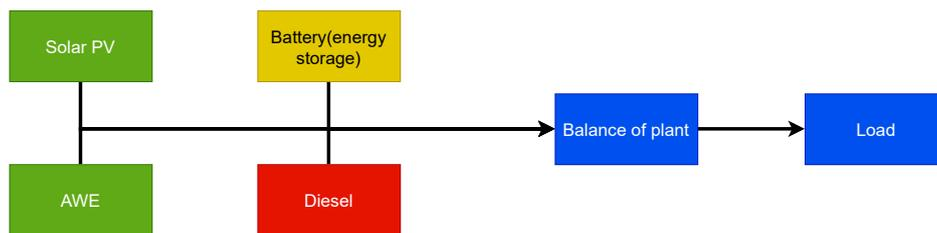
Figure 2.8: Simplified block diagram of a typical HPP
