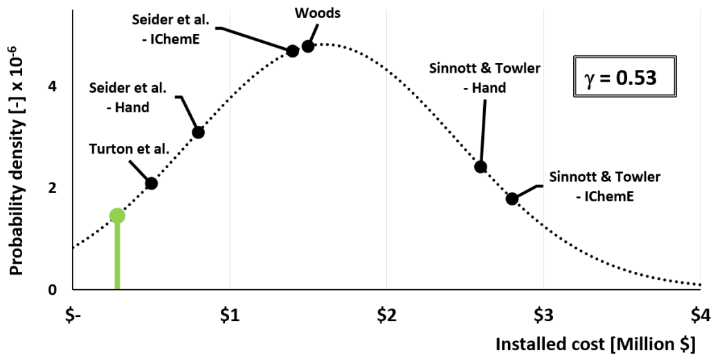
Figure U.8: The constructed normal distribution curve for case 3. The green line indicates the reference value.
