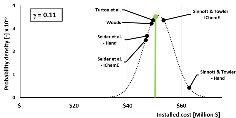
Figure 4.6: The constructed normal distribution curve for case 6 (NGL large). The green line indicates the reference value.
