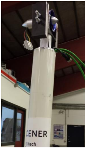
Figure 1. Former ducted fan actuator for the inclusion of the thrust as point force
