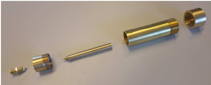
Fig. 1. Structure of the impedance probe.
