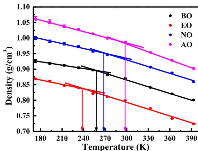
**Fig. 12.** The density variations of rejuvenators as a function of temperature.
