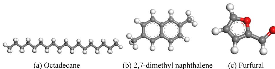
**Fig. 10.** The molecular elements in aromatic-oil rejuvenator.
