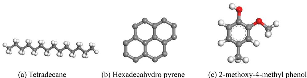
**Fig. 9.** The molecular elements in the naphthenic-oil rejuvenator.**Table 6**
