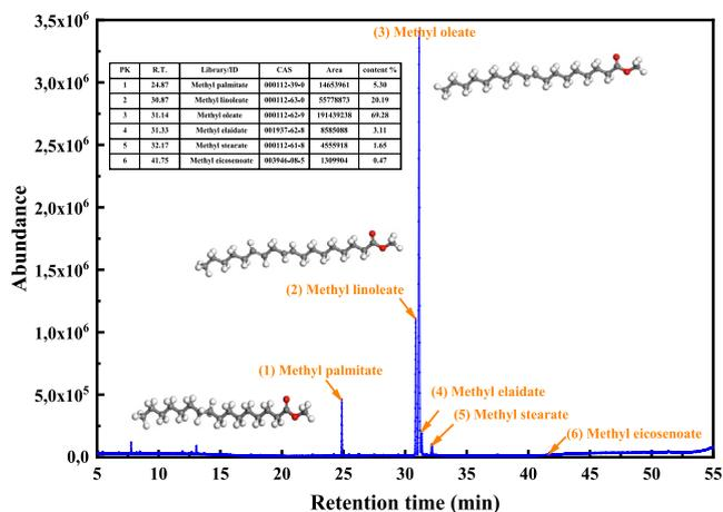
Fig. 3. The GC-MS curve of bio-oil rejuvenator.
