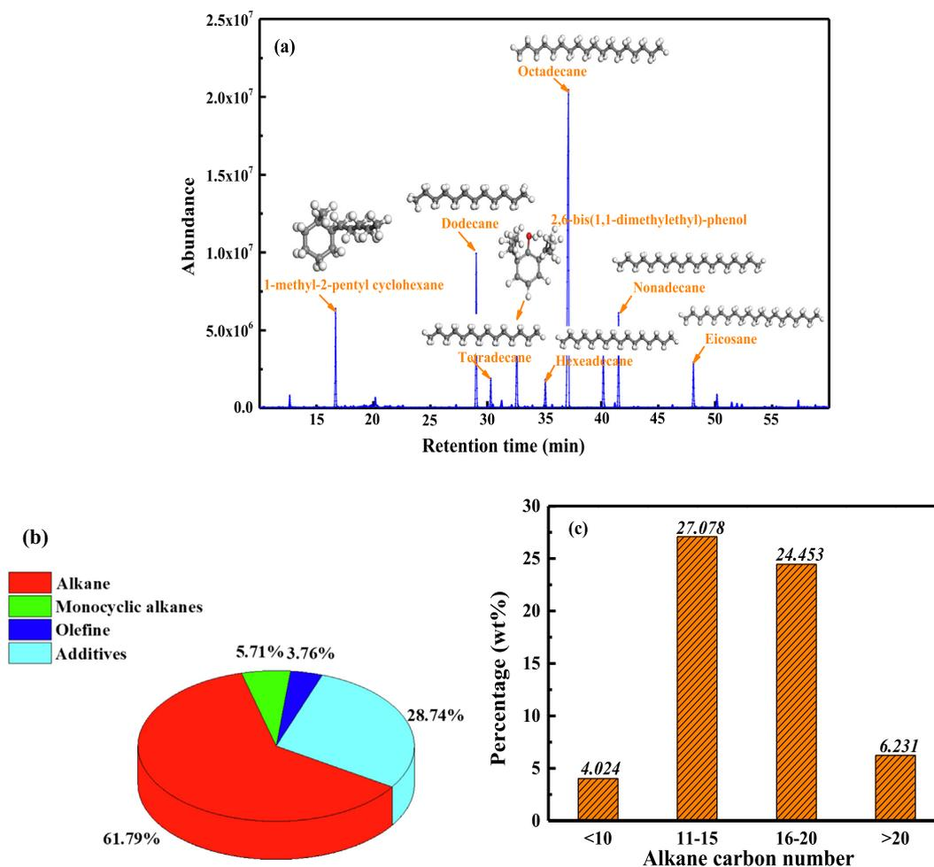
Fig. 4. The components distribution and alkane classification in engine-oil.
