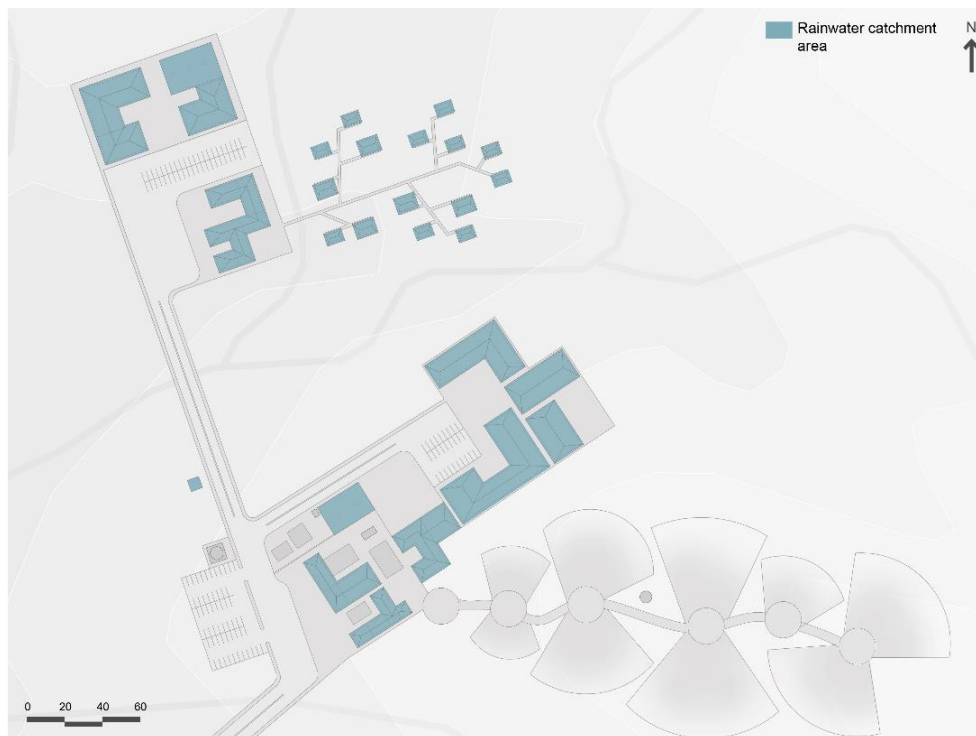
Figure 60: rooftops considered as catchment areas, (Author)
