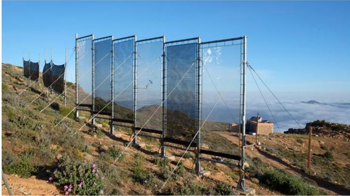
Figure 29: Image of an installed Fog harvesting device (Stenhouse, 2017)
