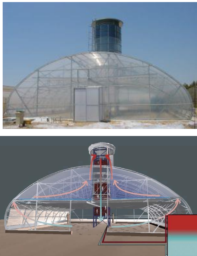
Figure 33: Image of the closed greenhouse (top) and section of the closed greenhouse indication airflow (bottom) ; (Buchholz, 2008)
