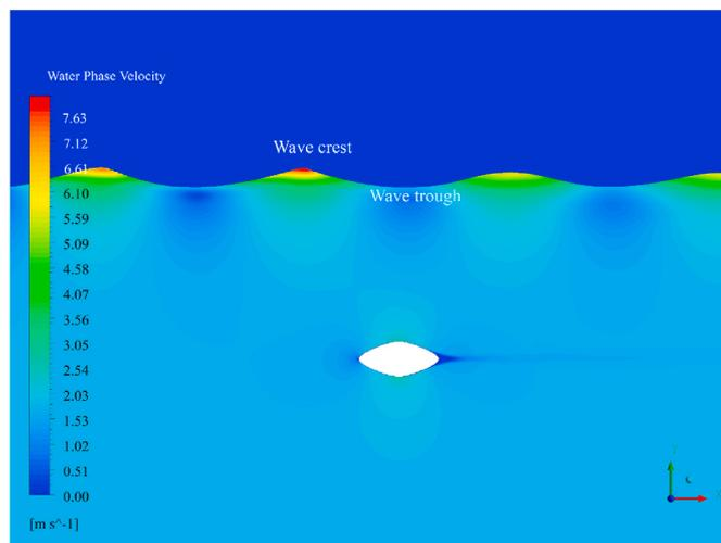
Fig. 19. Velocity contours around the SFT cross-section at  $t = 400$  s. The upper dark blue region is air, and the lower region is water. (For interpretation of the references to colour in this figure legend, the reader is referred to the Web version of this article.)
