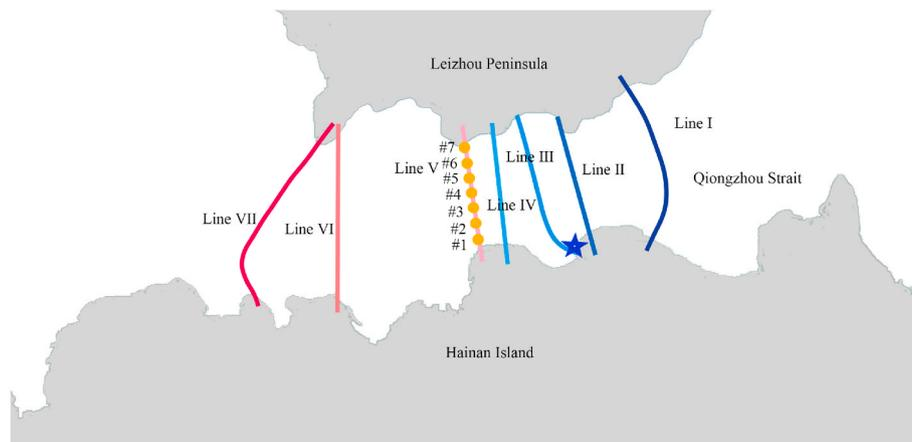
**Fig. 3.** The seven alternative headings for sea-crossing in the Qiongzhou Strait and the virtual gauge locations (yellow circles) along "Line V". The blue star denotes the observation station at Xiuying (110.34°E, 20.05°N) used for model validation. (For interpretation of the references to colour in this figure legend, the reader is referred to the Web version of this article.)
