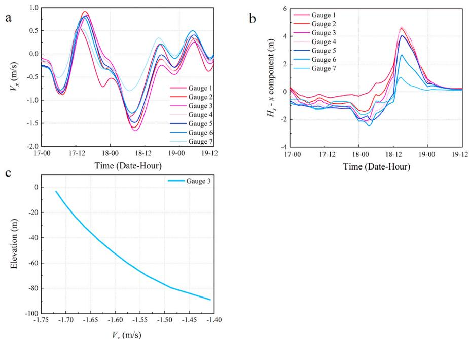
**Fig. 14.** Storm tide in the Qiongzhou Strait. (a) Along-strait depth-averaged current speed at the seven virtual gauges. (b) Along-strait wave height at the seven virtual gauges. (c) Vertical distribution of current speed when gauge #3 reached its maximum current speed value. x direction: positive to east and negative to west.
