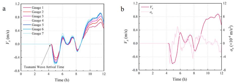
**Fig. 12.** Tsunami characteristics in the Qiongzhou Strait. (a) Current speed at the seven virtual gauges. (b) Current speed and acceleration at virtual gauge #7. x direction: positive eastward and negative westward.
