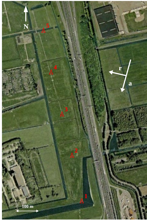
Figure 5.9: Delft CR experiment setup for ENVISAT ASAR descending acquisitions. CR and their numbers are marked in red as shown in the GoogleEarth (optical image date: 19-May-2004) (GoogleInc., 2017).
