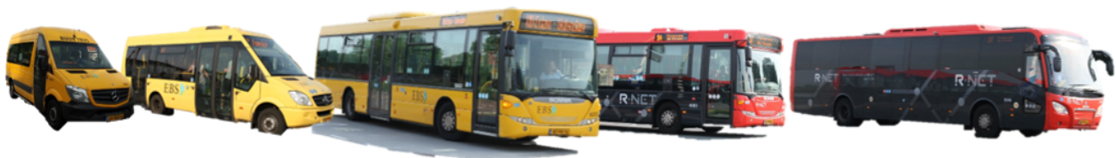
Figure 5.3: Equipment used in concession Waterland. From left to right: 8-person community service bus, 21-person midibus, 12m standard bus (both in regular and R-net branding (12.7m)), 18m articulated bus, Bizzliner touringcar.
