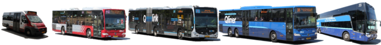
Figure 5.8: Equipment used in concession Groningen-Drenthe. From left to right: 8-person minibus, 12m standard bus, 18m articulated bus (both in regular and Q-link branding), Qliner touringcars (12m, 15m or double deck).
