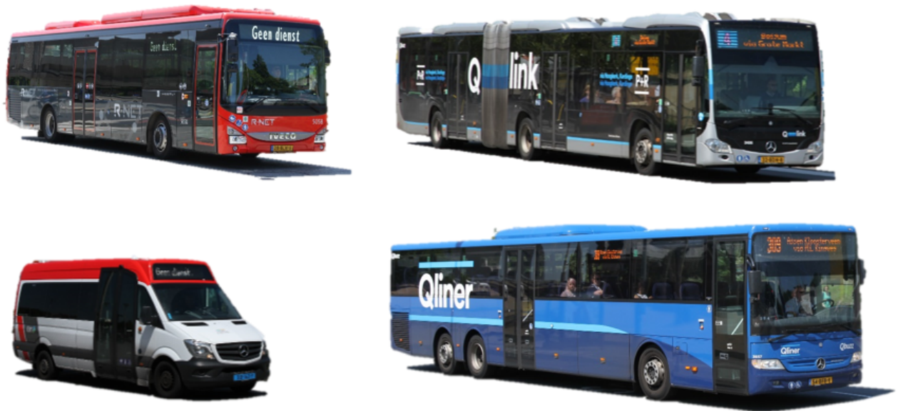
Figure C.1: Distinction between types of equipment used. Top left: 12m standard bus. Top right: high capacity (18m articulated) bus. Bottom left: 8-person vehicle/midibus (dependent on amount of seats). Bottom right: touringcar.
