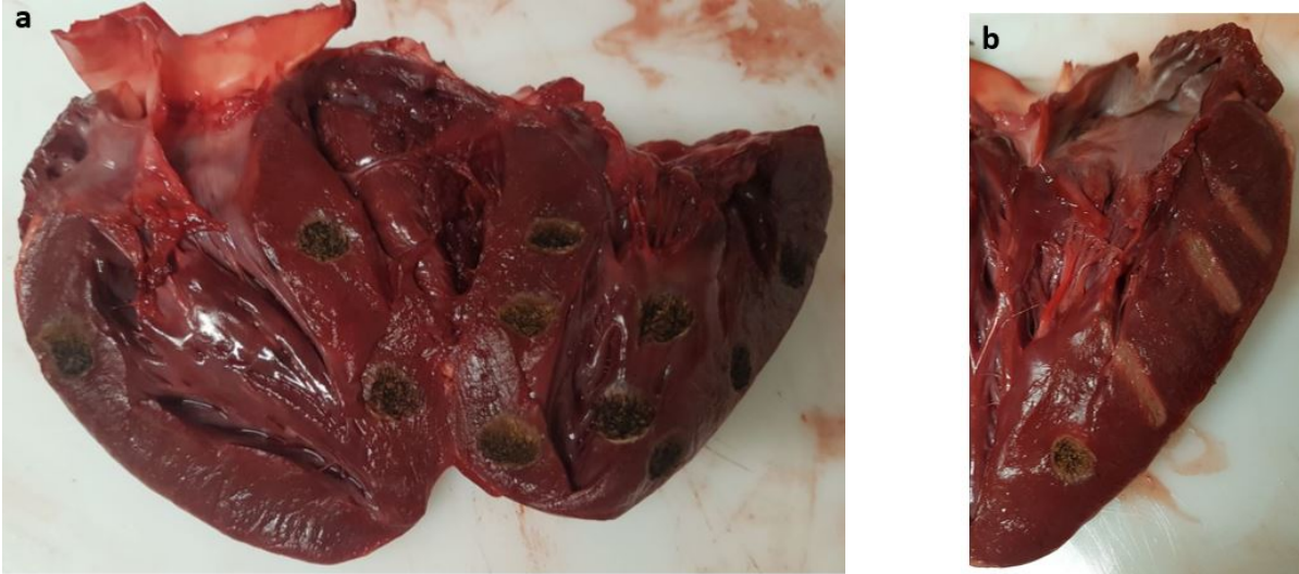
Figure H.1: Ablation effects of the fulguration (a) and the pure cut (b) modes
