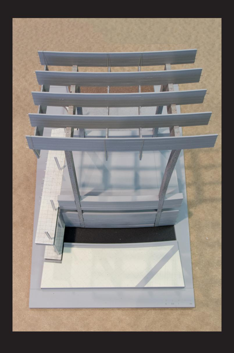
8. circular beams on top of portals, radial beams hung
