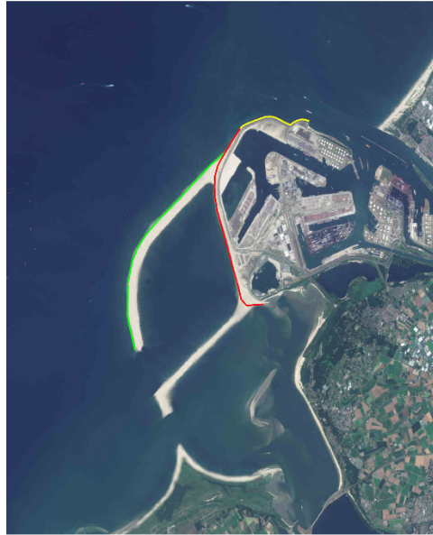
Figure 1.2: The research area of this thesis. The current soft sea defence of Maasvlakte 2 in red, the current hard sea defence in yellow and the to be researched soft sea defence of Delta21 in green.
