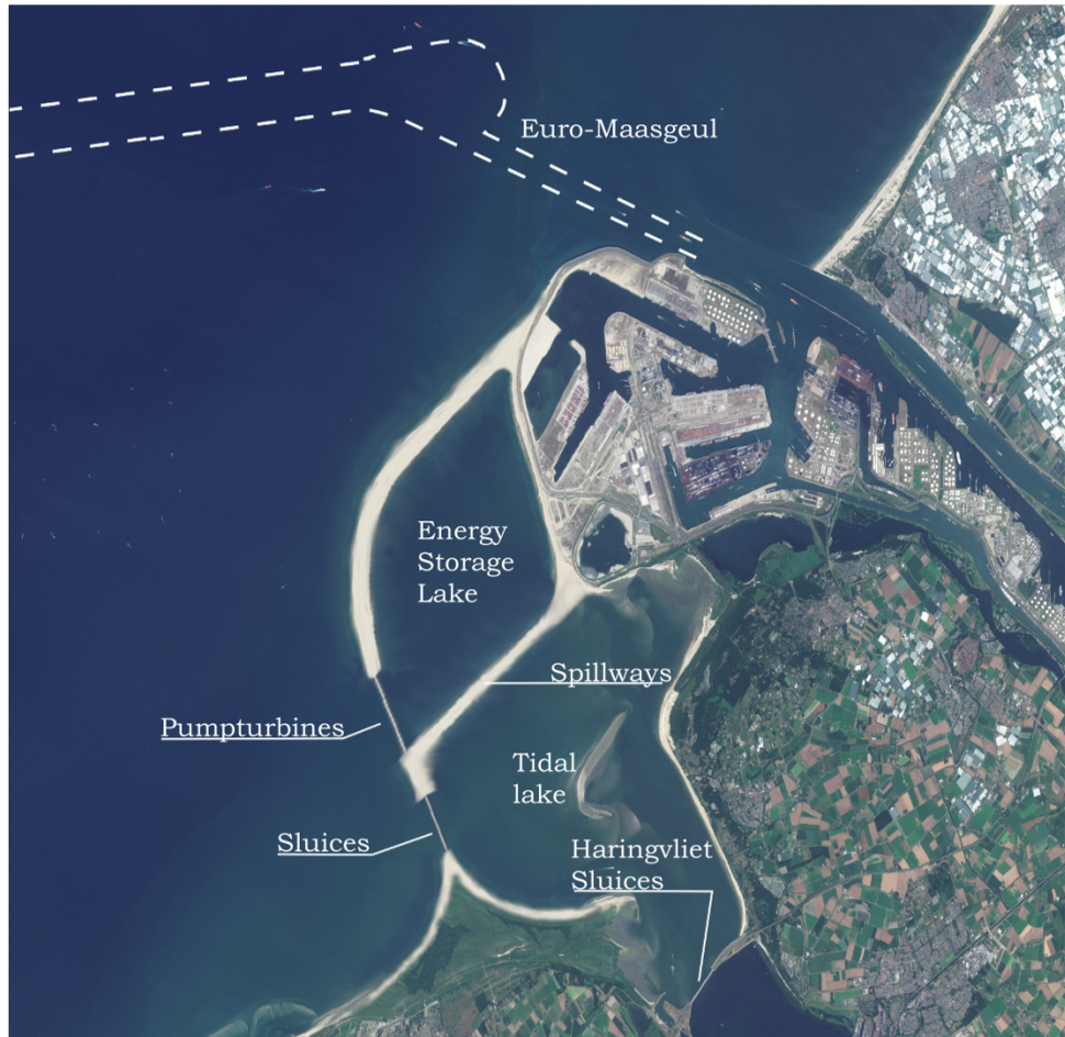
Figure 1.1: Delta21 project and its parts. Image: Sentinel2 - 10m resolution. 25-07-2019. Credits: European Space Agency (ESA)
