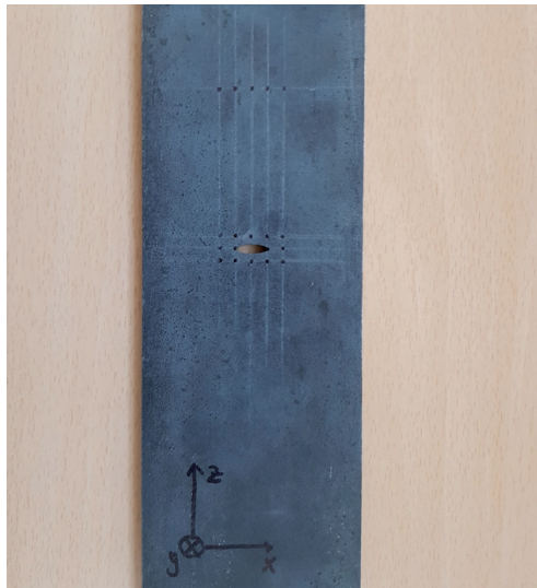
Figure 6.6: Test specimen with extra row of five measurement points 50 mm above elliptical hole.
