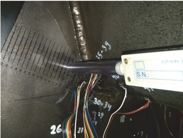
Figure 7.11: Measurement procedure with single axis magnetometer.
