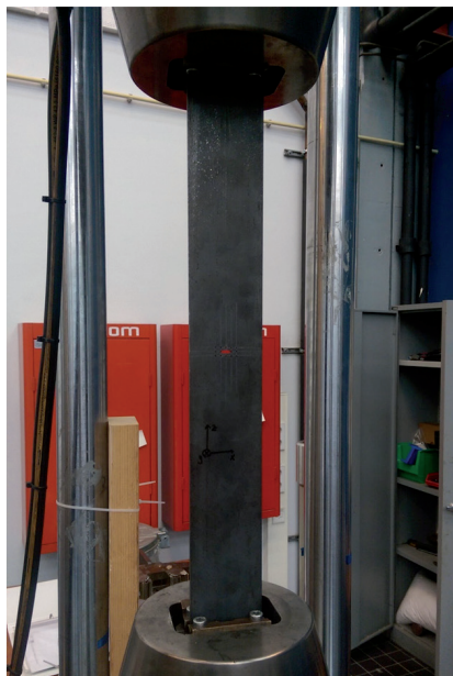
Figure 6.2: Specimen while clamped in the MTS fatigue testing machine.
