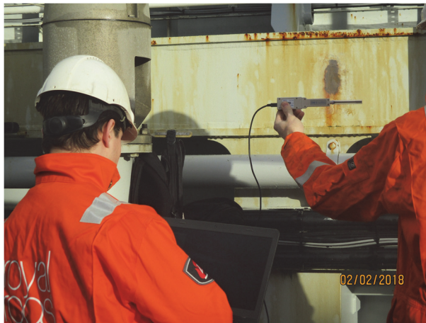
Figure 7.12: Measurement of background field in X-direction on suction hopper dredger.
