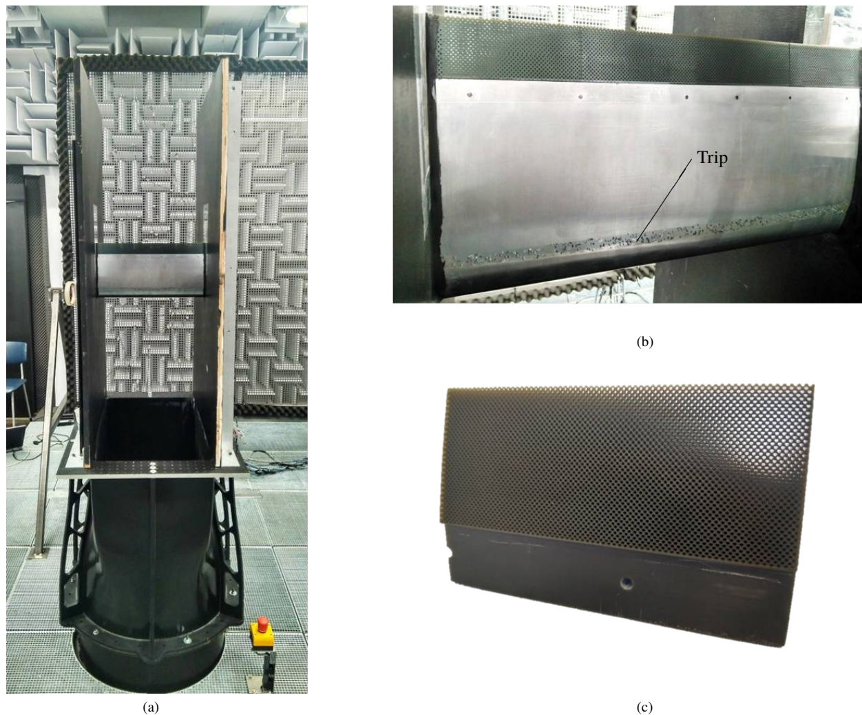
Fig. 2 (a) Overall view of the contraction with the airfoil and the side plates, and the microphone array on the back. (b) Detail view of the airfoil with a 3D-printed insert. (c) Detail of 3D-printed insert with l_h = 1.5 mm. Total length is 6 cm. Only the last 4 cm of insert are exposed to the flow.
