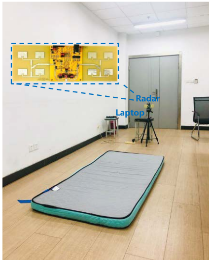
Fig. 6. Experimental setup with radar system and area where the activities are performed, including a mattress for controlled falls.
