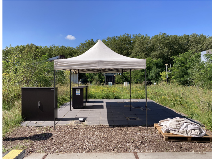
Figure 3.12.: Measurement set-up to analyse the effect of temporary shade.
