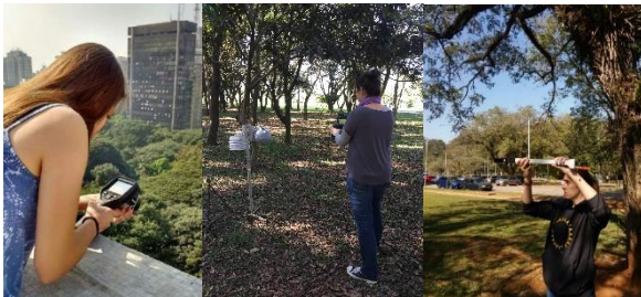
Figure 2: Fieldwork to measure surface temperature with a thermographic camera, air and surface temperature and air humidity in different locations and leaf area index with the canopy analyser.
