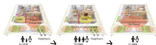
Figure 15: Example of partitions change depending on the family size. (a) Planning when the family has one child. The child room is placed at EN within eyeshot of parents. (b) Planning when the family number increase. Child rooms are placed in EN in order that neighbours can follow the children growth. (c) Planning after retired. The EN are opened to the neighbours to create the good relationship with community.
