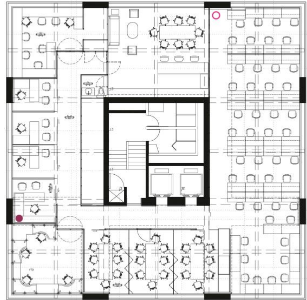
Figure 8: Existing layout of the 6th floor (after refurbishment), showing placement of dataloggers to record air DBT.
