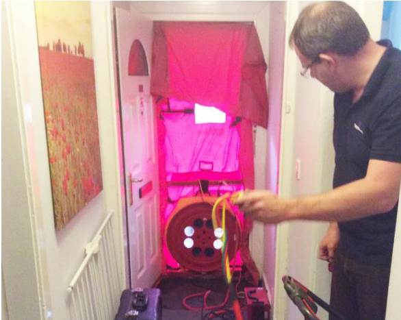
Figure 1: Airtightness tests are included in the basic BPE methodology, to quantify the impact of air leakages in the building fabric.
