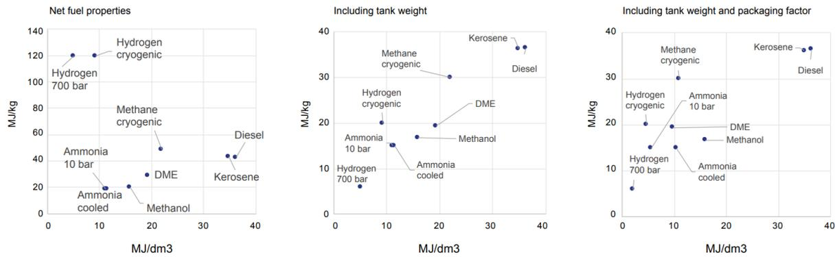
Figure 1: Energy density and specific energy of fuels with and without the tank weight and volume Van Kranenburg et al. (2020)
