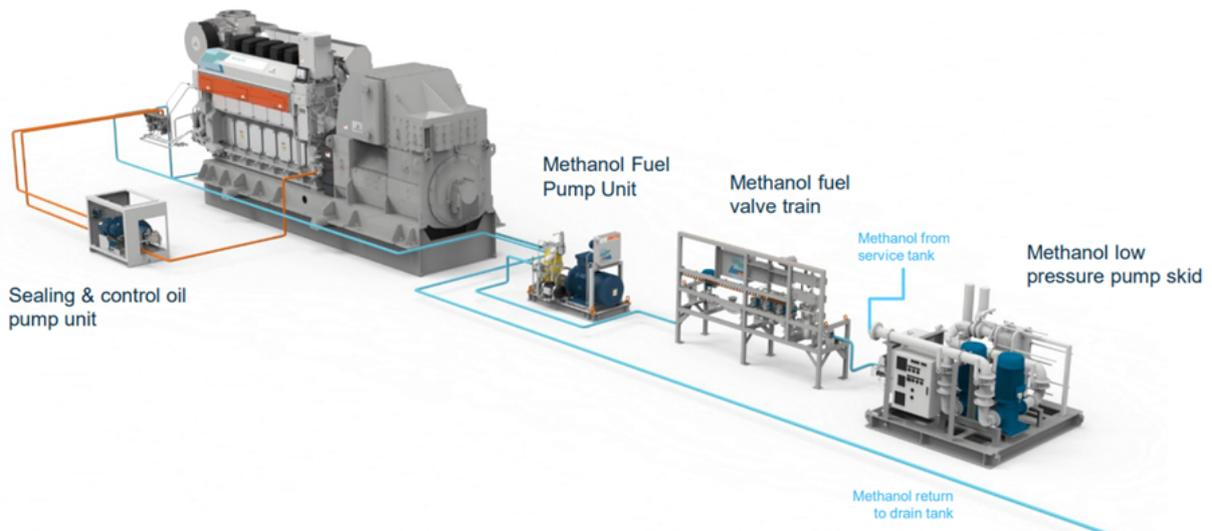
Figure 7: Wärtsilä W32 methanol engine system overview Wärtsilä (2022)
