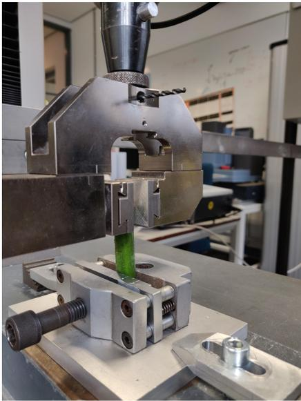
(a) A sample of the tomato plant is put in a tensile test bench to determine the Youngs modulus.
