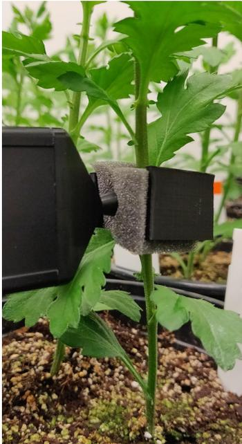
(a) Isolation (grey) between microphone and plant to dampen external noise, held in its place by a 3D printed clamp.
