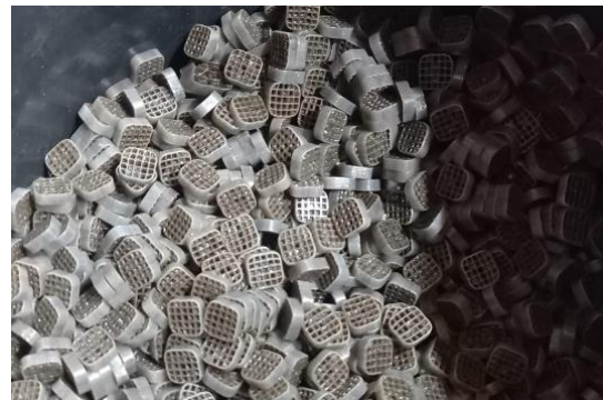
Figure 16: Picture of the used carriers in the MBBR reactor
