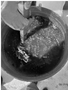
Figure 13: Picture of the flocculation by the CP314 conditioner on BW
