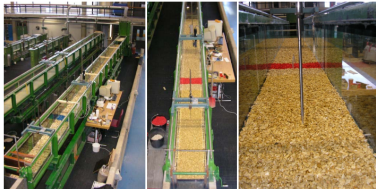
Figure 4.1: Flume with test set-up in the Environmental Fluid Mechanics Laboratory (Van de Sande, 2012).
