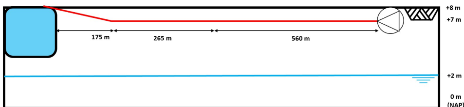
Figure 11.18: Schematic overview of pipeline situation side
