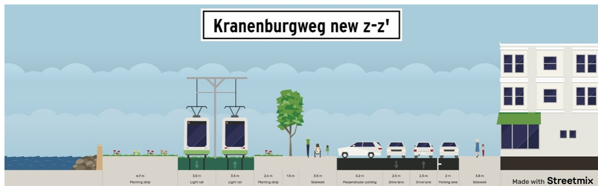
Figure 12.14: Kranenburgweg section Z-Z' in the new situation (Gemeente Den Haag, 2015)
