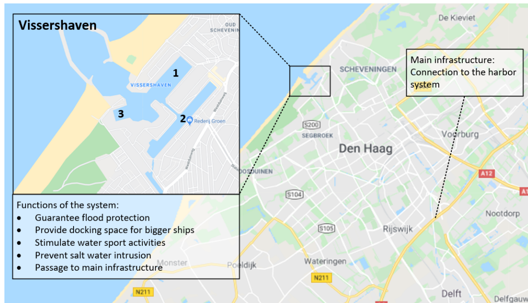
Figure 2.7: Schematic overview of the different functions of the system. Numbered are the current harbors already existing (OpenStreetMap contributors, 2017)
