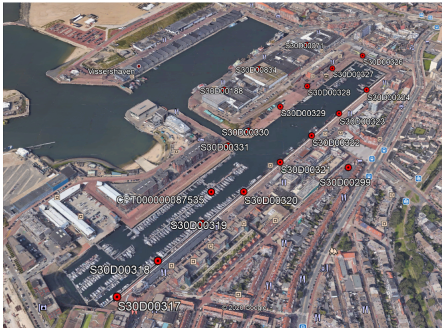
Figure D.14: Available conus penetration tests locations. One can see that there are multiple which might be representative for the potential location for the compression pile. Important is that data starting with 'S30' was made available by DINO, while data starting with CPT was made available by BRO.
