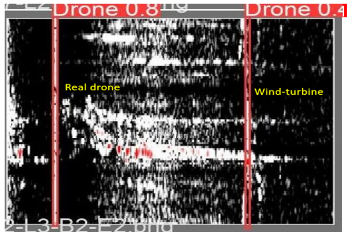
Fig. 4. Example of output of the proposed model, with detections obtained using SGD optimizer. A false alarm induced by a wind turbine is reported, together with a true detection.
