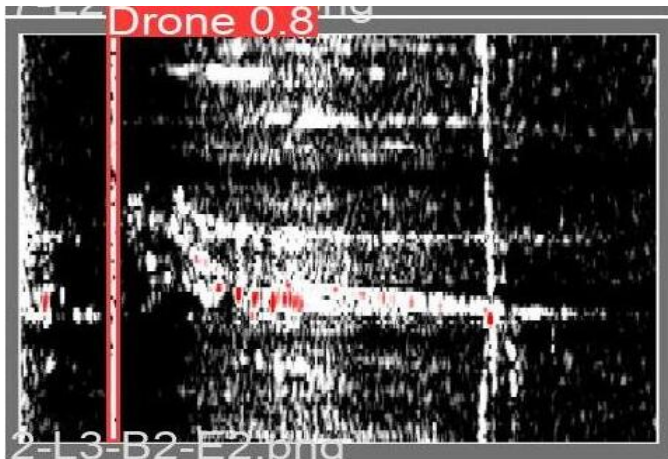
Fig. 6. Example of output of the proposed model for the same range-Doppler plot of Fig. 4 and 5, but using SGD optimizer and genetic algorithm. The genetic algorithm combined with SGD did not yield false detections.
