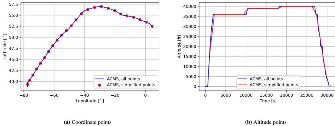
**Figure 6:** Complete and simplified trajectory points, for the flight KL0651 Washington D.C. (KIAD) - Amsterdam (EHAM) on 25-09-2021
