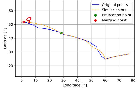
Fig. 6. Example of similar trajectories found by the Pairing method of Experiment 1 for a flight VIDP-EGLL (Delhi-London)
