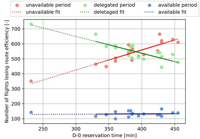
Fig. 22. Number of flights losing route efficiency in the Delta sector from the Pairing method of Experiment 1, per time reserved and period of hypothetical FUA transit
