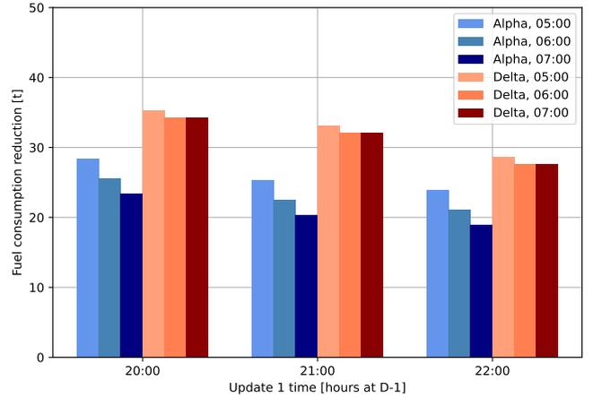
Fig. 19. Fuel consumption reduction of the AUP Updating concept per combination of AUP update times
