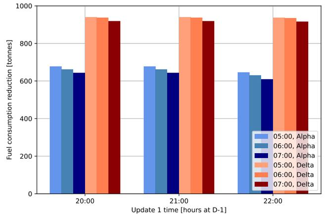
Fig. 20. Fuel consumption reduction due to tactical route efficiency benefits enabled by the AUP Updating concept
