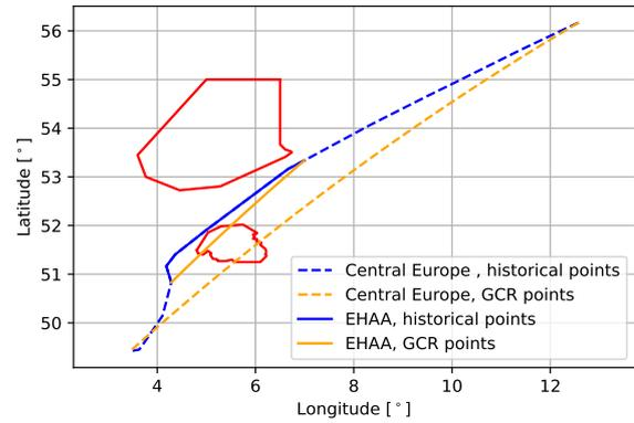
Fig. 5. Historical and GCR trajectory segments for a flight RKSI-LFPG (Incheon-Paris), limiting the GCR to EHAA and Central Europe
