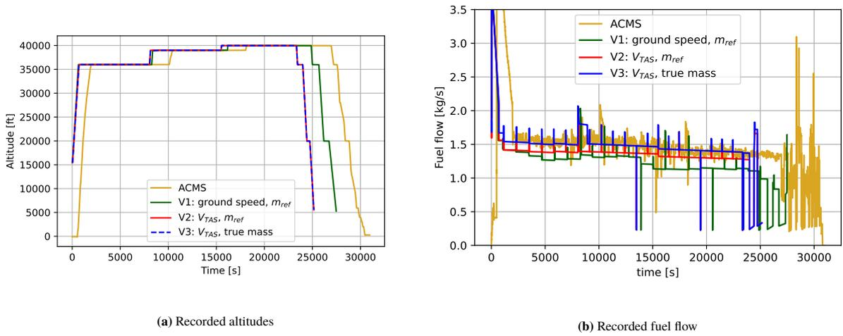
**Figure 8:** Altitude and fuel flow data as simulated by BlueSky, for the flight KL0651 Washington D.C. (KIAD) - Amsterdam (EHAM) on 25-09-2021
