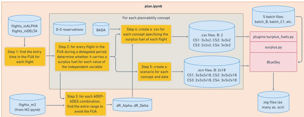
Figure 17: Main parts of the `plan.ipynb` script, used for Experiment 2
