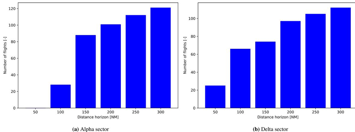
**Figure 6.1:** Effect of the range (distance horizon) from the FUA at which the GCR is enabled on the number of flights benefiting from traversing the FUA. Note that for this, all flights are considered regardless of the period they would have transited the FUA.
