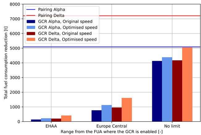
Fig. 14. Experiment 1 results: total fuel consumption reduction
