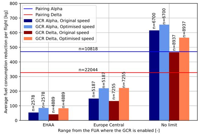
Fig. 13. Experiment 1 results: average fuel consumption reduction per flight
