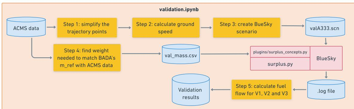
**Figure 21:** Main components of the script validating the fuel flow calculation under the experiment assumptions (validation.ipynb)
