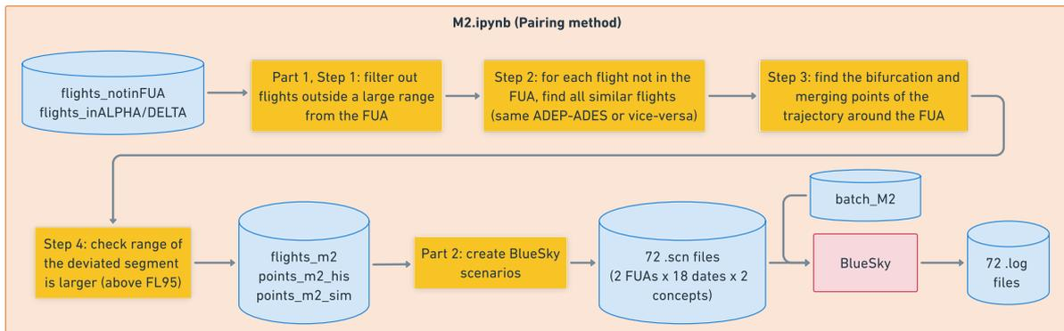
Figure 15: Main parts of the M2.ipynb script, the Pairing method of Experiment 1
