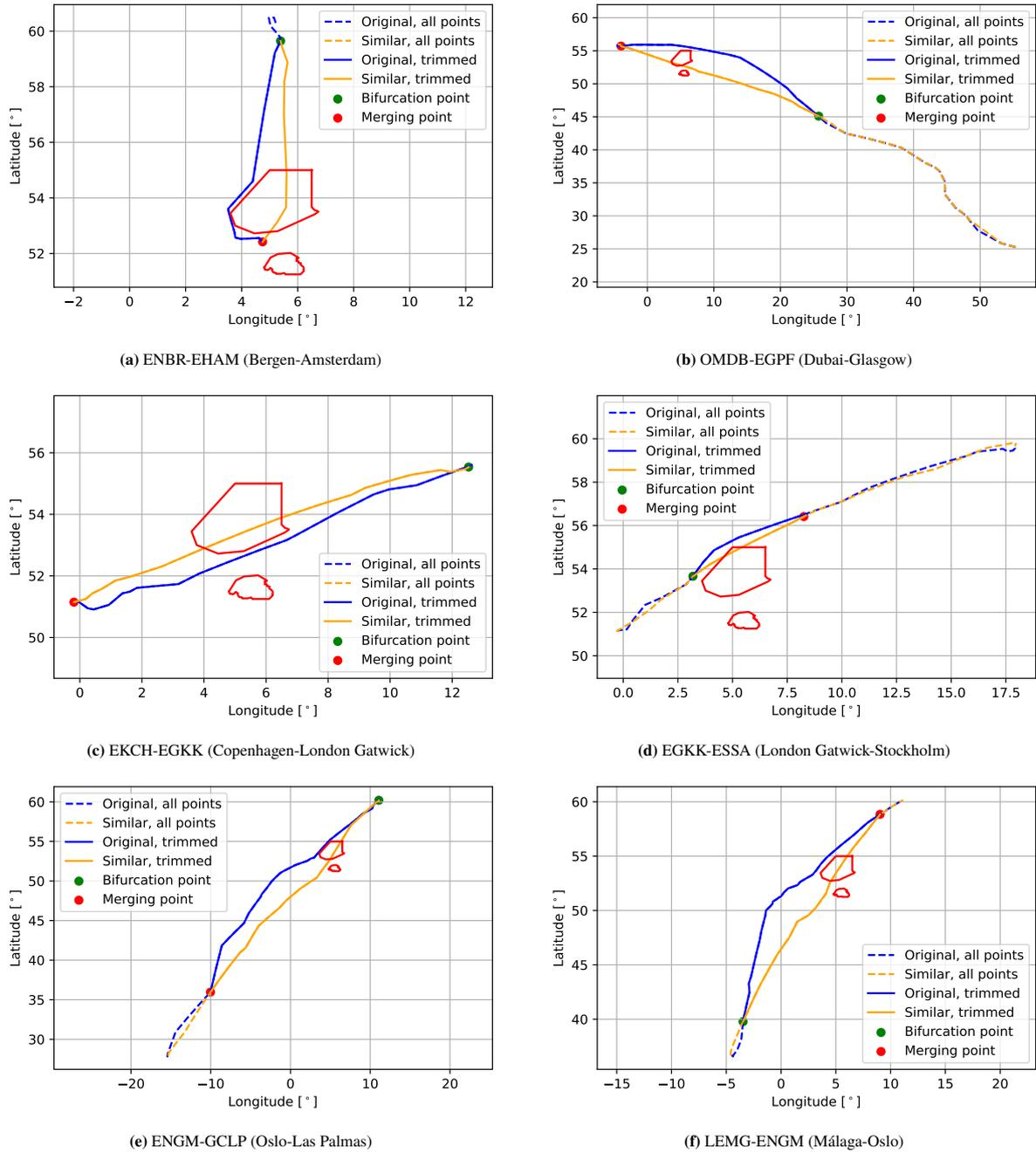
**Figure 25:** Examples of flights found by the Pairing method to traverse the Alpha sector
