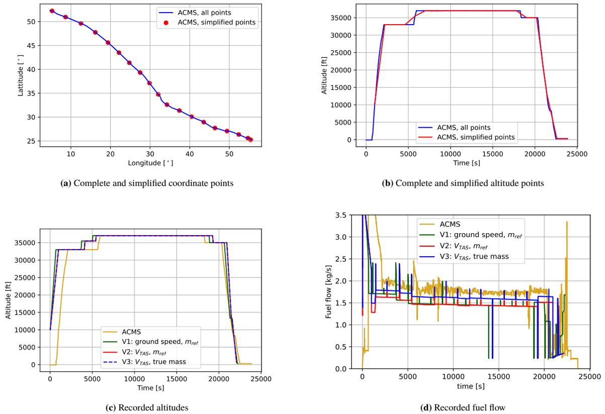
**Figure 11:** Simplified points and simulation results for the flight KL0427 Dubai (OMDB) - Amsterdam (EHAM) on 18/09/2021
