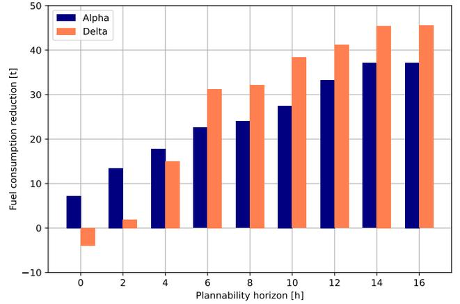
Fig. 16. Fuel consumption reduction of the Single Horizon concept per planning horizon
