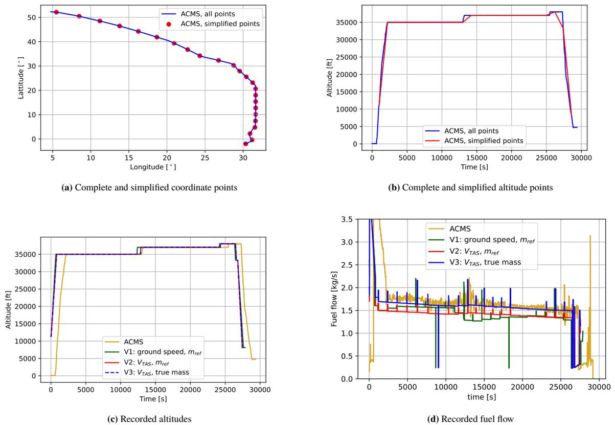
**Figure 10:** Simplified points and simulation results for the flight KL0535 Amsterdam (EHAM) - Kigali (HRZR) on 15-09-2021
