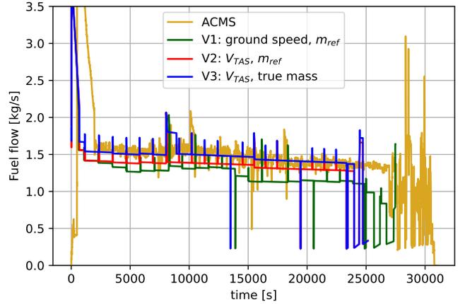
Fig. 25. Fuel flow validation for Airbus A-330
