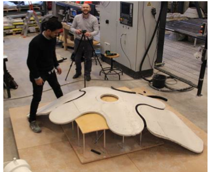
Fig. 22. Assembly of final shell.
