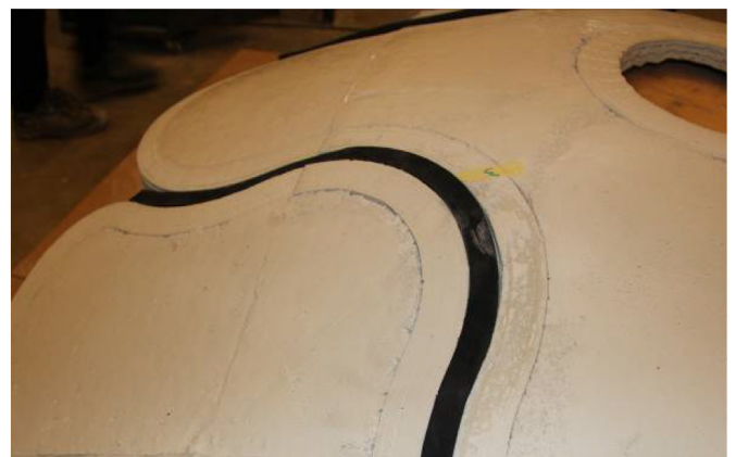
Fig. 23. Seam between two panels indicating a tight fit.
