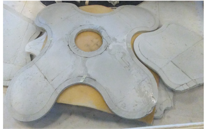
Fig. 21. Demolded final pavilion.
